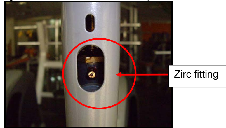
Fig. 2. Lubrication mode stride motor position
